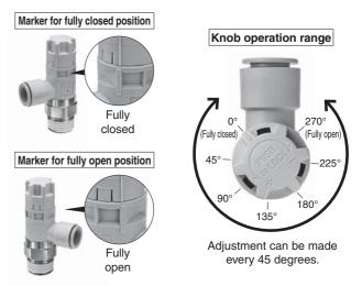
6. Do not use tools such as pliers to rotate the knob. It can cause idle rotation of the knob or damage.
