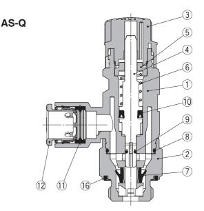
Air Saving Speed Controller For R, NPT thread AS-R/AS-Q Series
