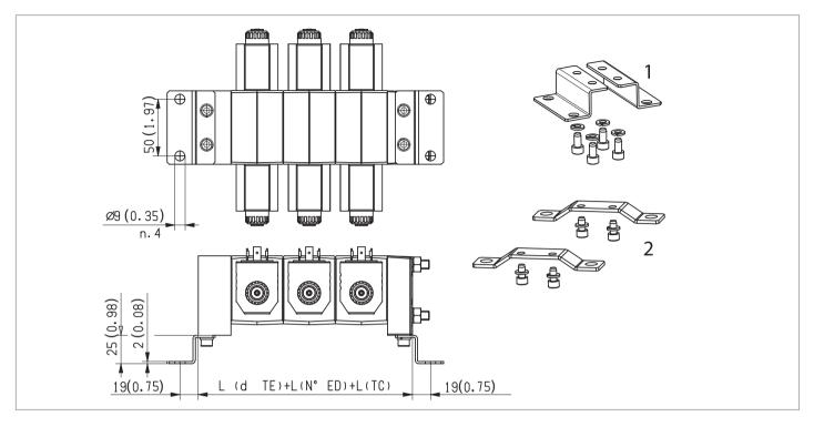
The kit is composed by 2 brackets, 4 screws and 4 washers.
