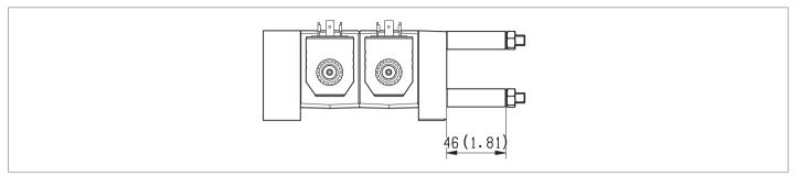
The spacers (code 44-00257012) are fitted in order to install longer tie-rods for future insertion of an extra directional element.
