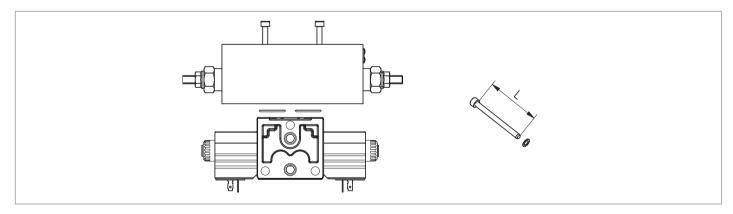
The assembly kit is composed by 4 screws and 4 washers.
