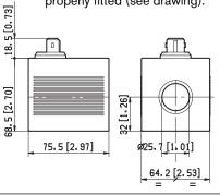
With coils having bi-directional diode and bipolar sheathed free lead, 350 mm long, without pins.
