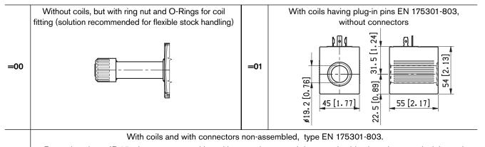
Protection class: IP 65 when connector with seal is properly screwed down, and cable clamp is correctly tightened.
