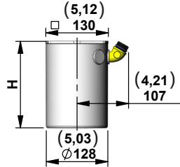
For this tanks is necessary to use the O-RING Ø112x3
