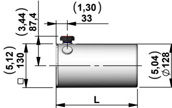
For this tanks is necessary to use the O-RING Ø112x3
