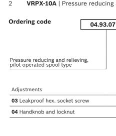
Z 00 Series 0/A to L unchanged performances and dimensions Version and options standard **SPRINGS** Std. setting Adj. press. range Pressure increase bar (psi) bar/turn (psi/turn) bar (psi) (reduc mode) 05 25-100 (360-1450) 31 (450) 50 (725) for 48 (696) 10 35-140 (500-2000) 100 (1450) X= 03 20 70-280 (1000-4000) 88 (1276) 200 (2900) for 35 35-350 (500-5000) 68 (986) 350 (5000) X = 04
